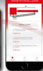
3. The App automatically calculates the position dimensions of the brackets
